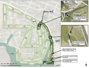
the clubhouse and at green #1. The additional surface course will add approximately 3" of height to the path, and will be backfilled and seeded to maintain a smooth transition. In between holes #3 and #4, certain portions of the cart path will be converted from decomposed granite to either limestone or asphalt.
