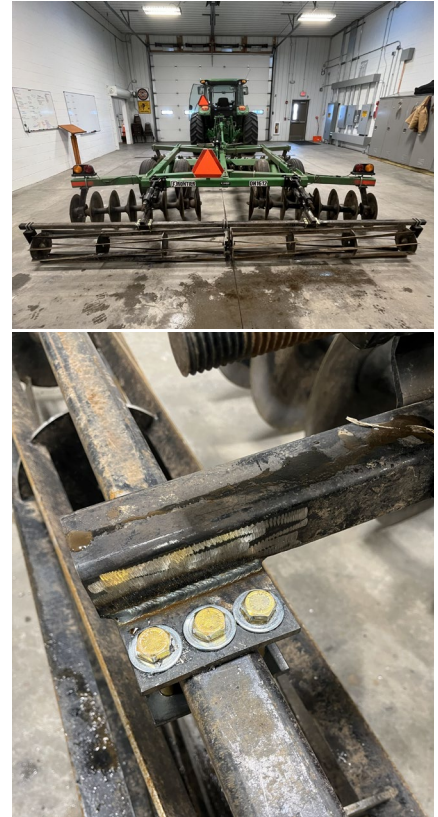
Photos of the disc attachment welding completed by Mechanic Tyler Rowe.
